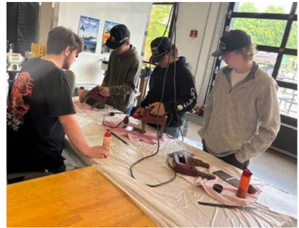
Students learning how to test welds using a magnetic particle tester.
