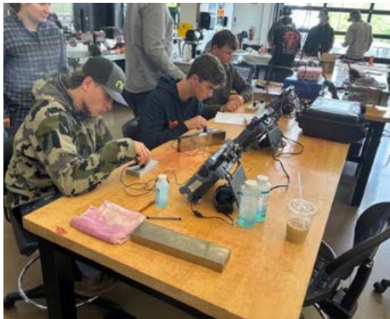
Students learning how to use ultrasound to test for weld defects
